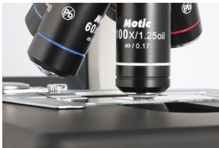
▲ Objectives with a small working distance (40X, 60X) are mounted close to the 100X lens and thus take the greatest risk for contamination with immersion oil from the slide surface. A preventive maintenance is recommended for these objectives.
